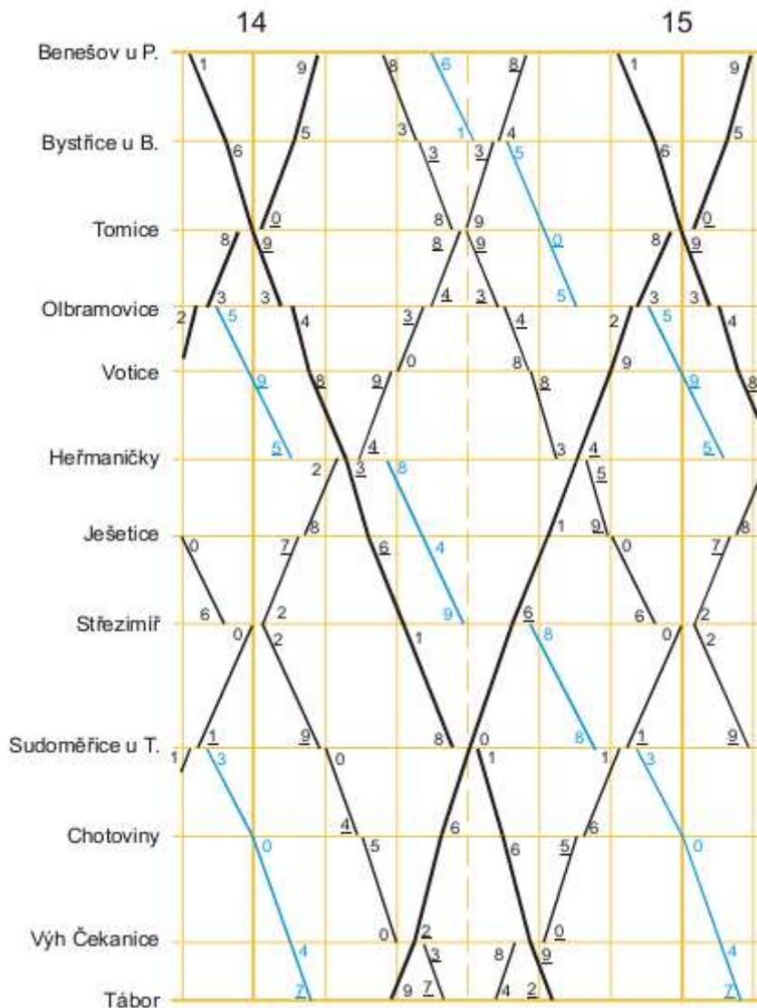
**Figure 2.7** PFTPs on single-track line. Contrary to periodic passenger timetable, these PFTPs cannot be scheduled into zero symmetry with PFTPs in opposite direction, because they are designed to pass through outside stations exactly at zero minute. (Kryže 2005).
