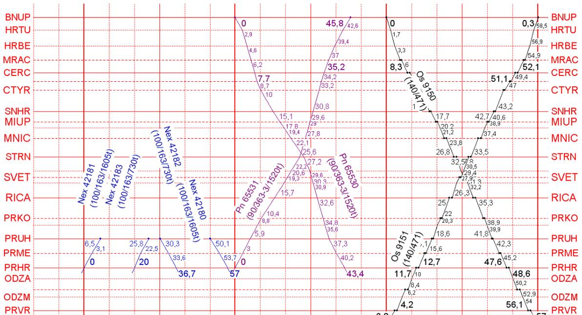
**Figure F.2** Train diagram of model freight trains on the line 519A/221, section Benešov u Prahy – Praha-Hostivař.
