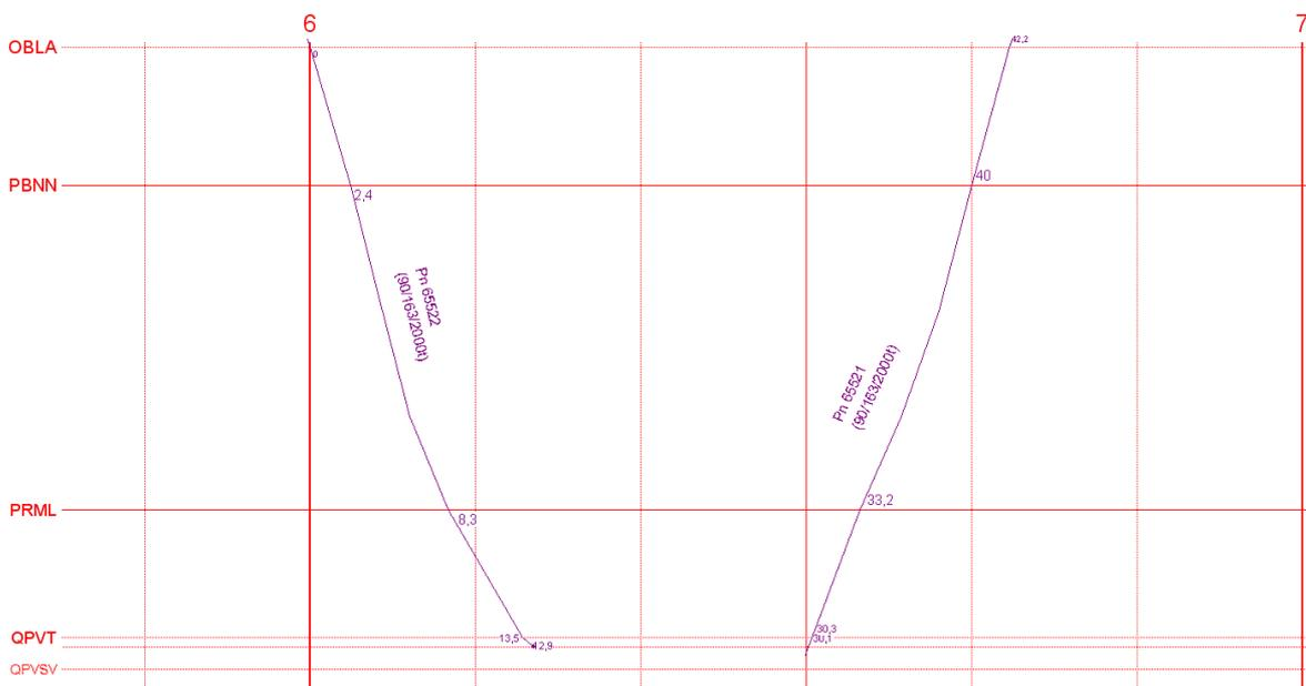
**Figure F.6** Train diagram of model freight trains on the freight bypass line 525G, section Odb. Blatov (part of the station Praha-Běchovice) – Praha-Malešice – Praha-Vršovice čekací koleje.
