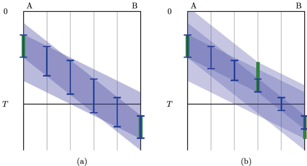
**Figure 1.1** Illustration of slot propagation in line section with 2 (a) and 3 (b) stations with restricted time windows for running of a train ([Caimi et al. 2009b](#)).
