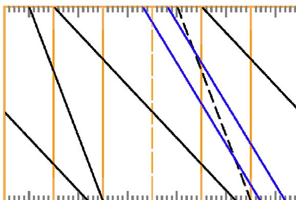
**Figure 2.11** Illustration of a conflict between PRUs' and FRUs' requirements for railway capacity allocation.
