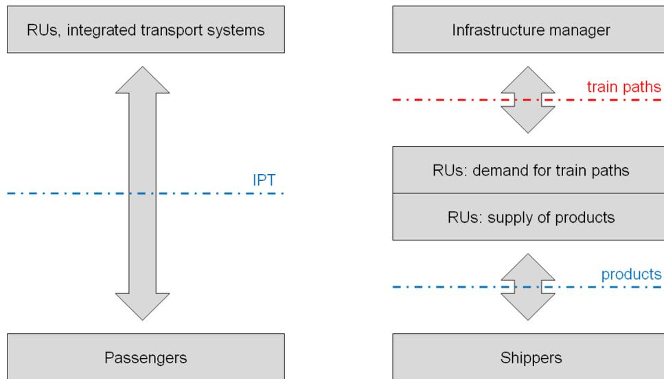
**Figure 3.7** Interface between offer and demand in the case of IPT (passenger services ordered by public sector) and liberalised freight railway.
