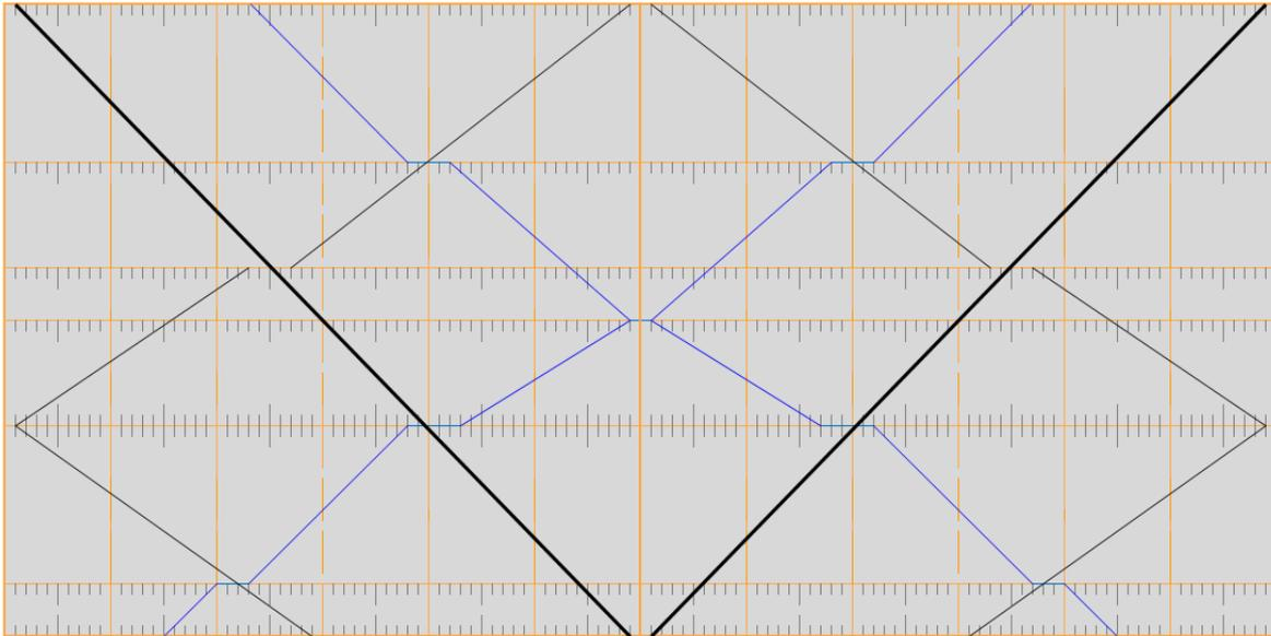
**Figure 3.17** Construction of PFTPs on single-track line with two segments of passenger transport (each with 120 min period).
