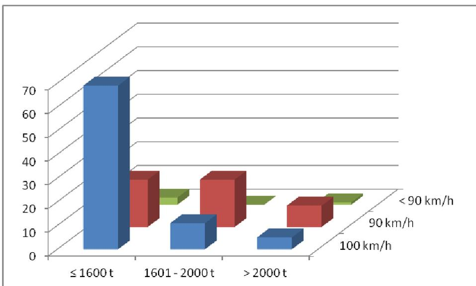
**Figure 3.2** Numbers of freight trains, scheduled through station Tlumačov – overall 138 trains. 87% of them can run at 90 or 100 km/h and their brutto mass of load does not exceed 2000 t. Data: [SŽDC \(2009b\)](#)
