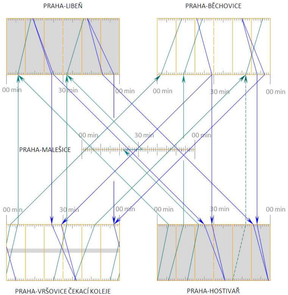
**Figure 4.2** Node diagram of station Praha-Malešice and neighbouring sections. Accented line stands for PFTP available only outside passenger peaks. Passenger train paths are not depicted. Direction north → south is marked with blue colour, direction south → north with turquoise colour.
