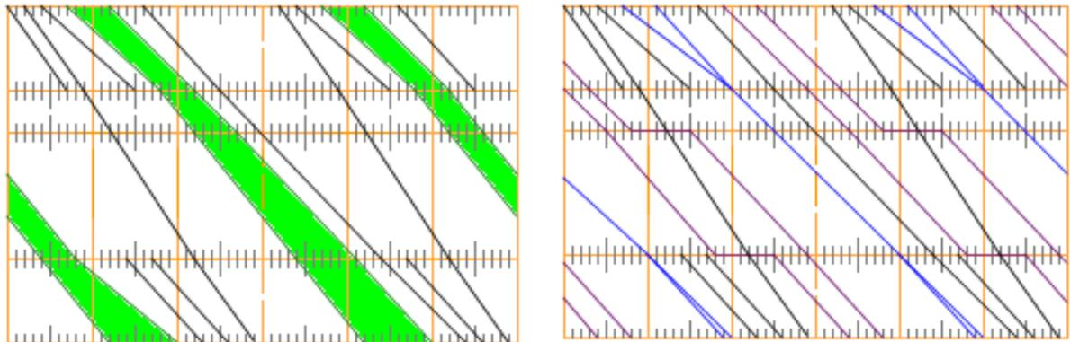
**Figure 3.10ef** Marking of capacity for passing of a freight train through whole line without stop and construction of priority PFTPs (with alternative connection from/into more directions) and local PFTPs.
