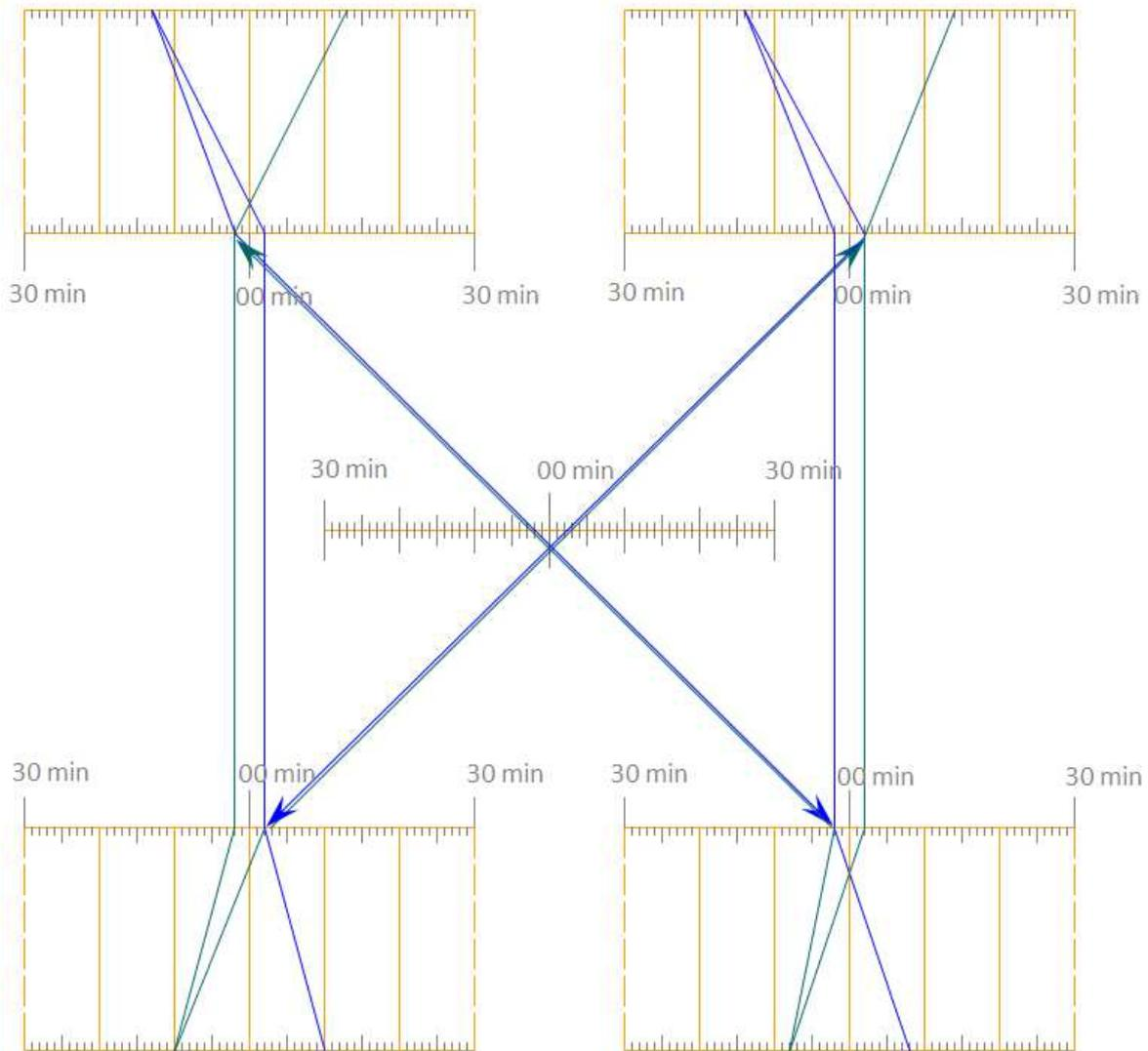
**Figure 3.14** An ideal freight IPT-node depicted by node diagram. Type of station is the same as in Figure 3.13. Direction north → south is marked with blue colour, direction south → north with turquoise colour.
