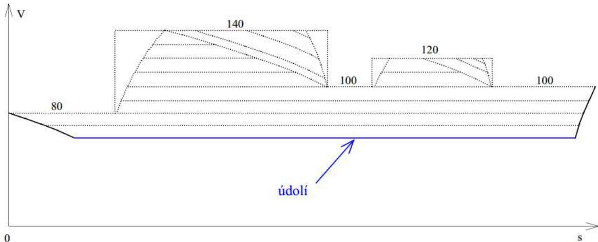
**Figure 3.8** Utilisation of “coasting valley” (marked by blue colour) for few minutes lengthening of runtime. (Vicherek 2011)
