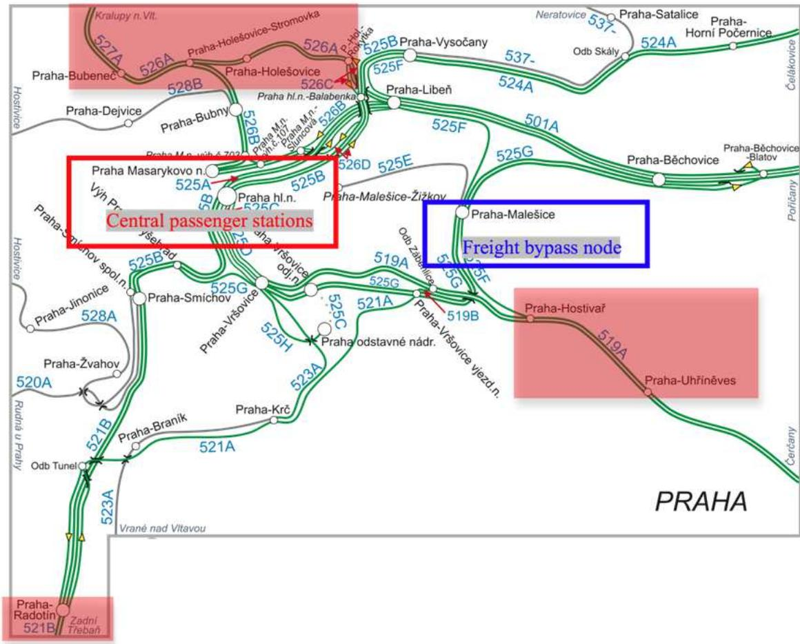
**Figure 4.1** Prague node area – main track layout plan (Drábek 2011). The author marked bottlenecks (pink colour) and significant stations. The number of trains per hour was comparatively low (Table 4.1), but, on the other hand, some stations and block posts were equipped with mechanical interlocking and two stations on double-track lines have at-grade access to platforms (Praha-Bubeneč, Praha-Hostivař). Map source: SŽDC (2008).
