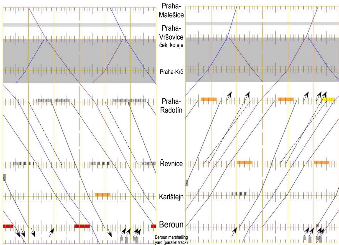
Figure I.3 Proposed train diagram of PFTPs for the line 512A/171.
