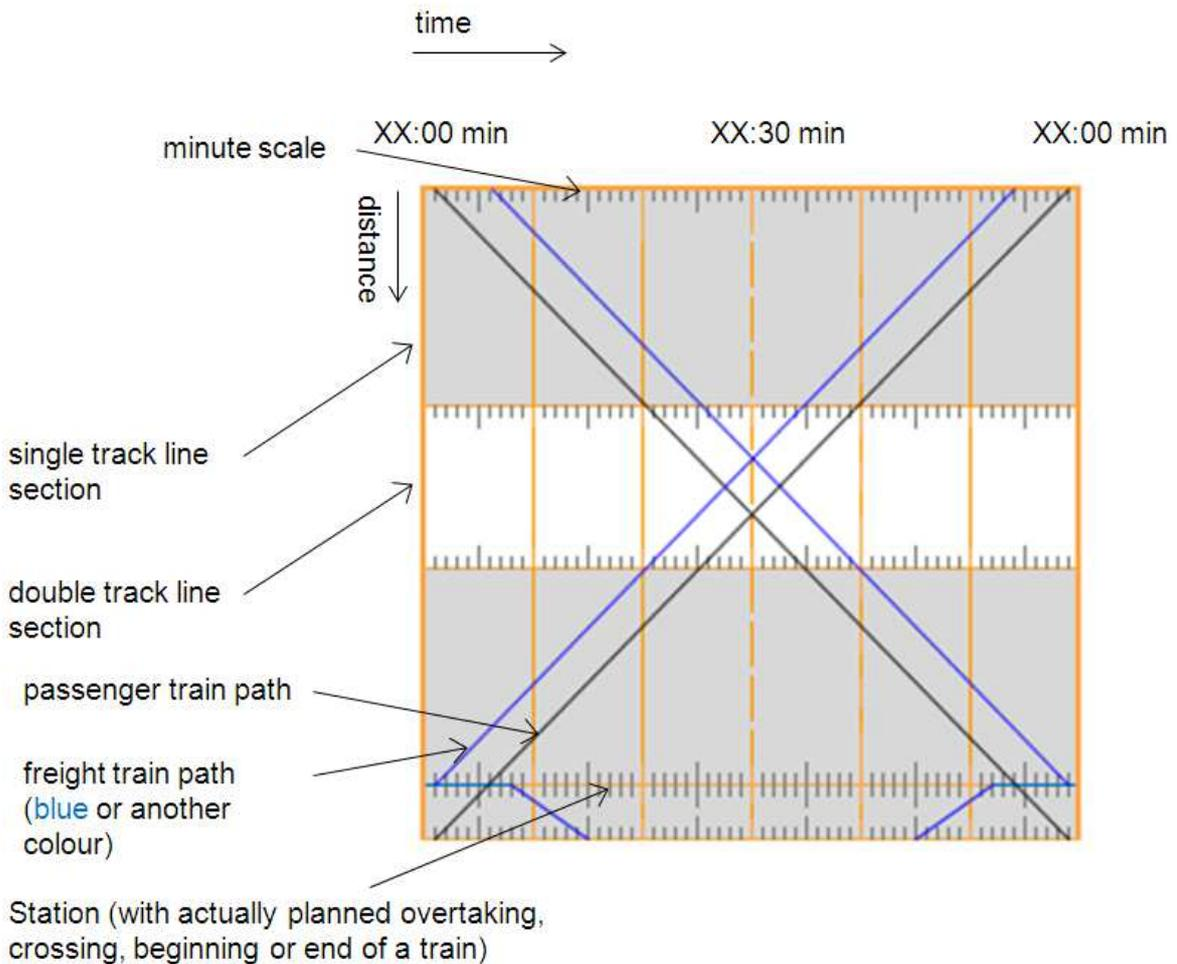
**Figure 1.3** Usual depiction rules of a fictious or real, but simplified train diagram in this thesis.
