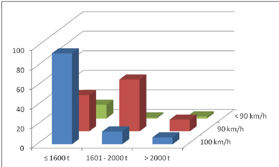
**Figure 3.1** Numbers of freight trains, scheduled through station Polom – overall 232 trains. 84% of them can run at 90 or 100 km/h and their brutto mass of load does not exceed 2000 t. Data: [SŽDC \(2009b\)](#)
