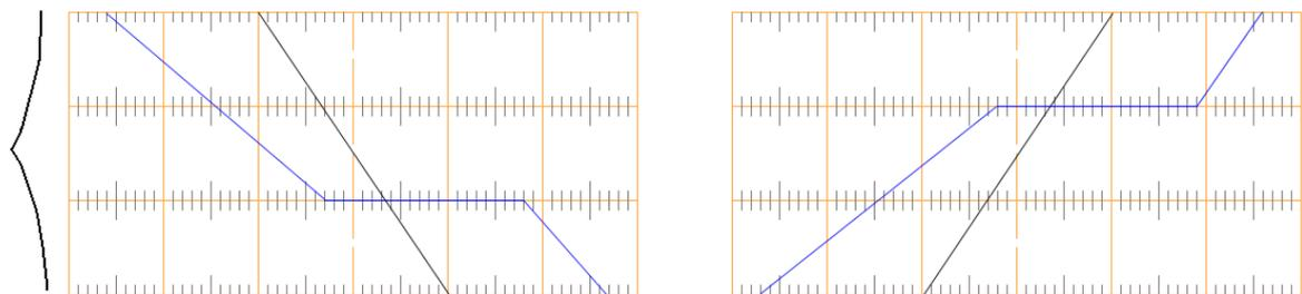
**Figure 3.11** Local asymmetry, but global zero symmetry of PFTPs on fictious double-track line with peak in the middle. Altitude profile of the line is marked left.
