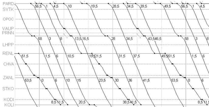
**Figure 4.7** Part of train diagram Pardubice – Kolín (one direction). Passenger timetable is planned without regard to freight transport (Kopecký et al. 2009, Drábek and Záruba 2010b).
