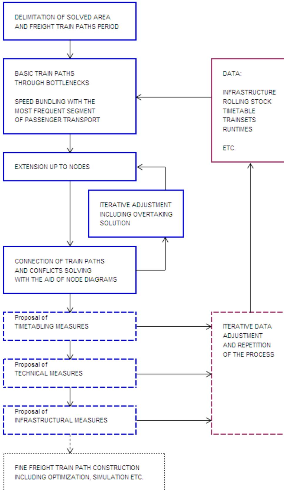
**Figure 3.15** Framework process for construction of network-bound periodic freight train paths.
