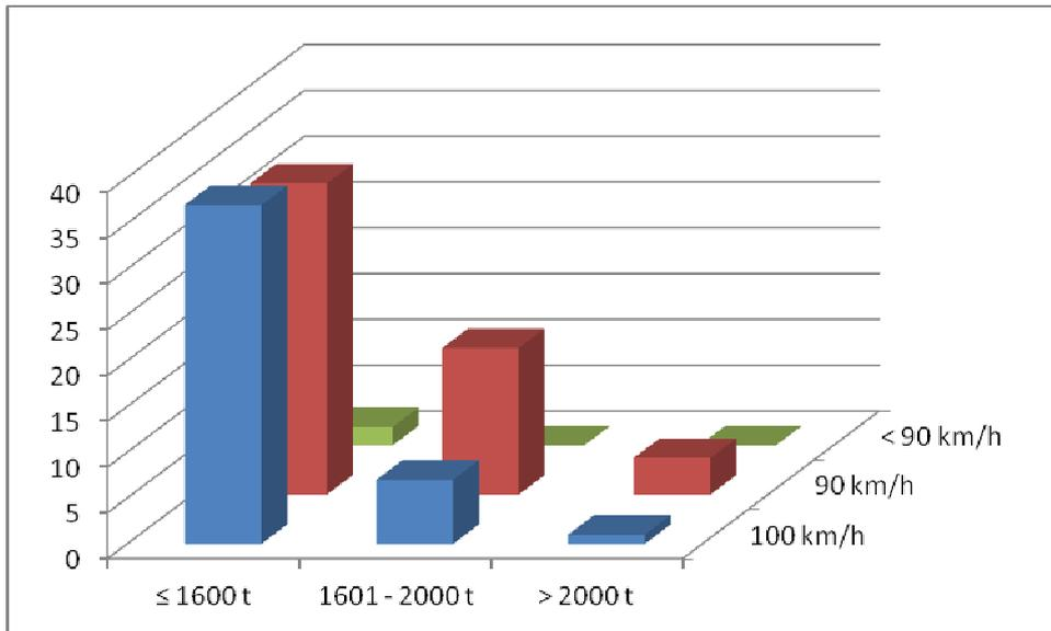
**Figure 3.3** Numbers of freight trains, scheduled through station Úvaly – overall 101 trains. 93% of them can run at 90 or 100 km/h and their brutto mass of load does not exceed 2000 t. Data: [SŽDC \(2009b\)](#)
