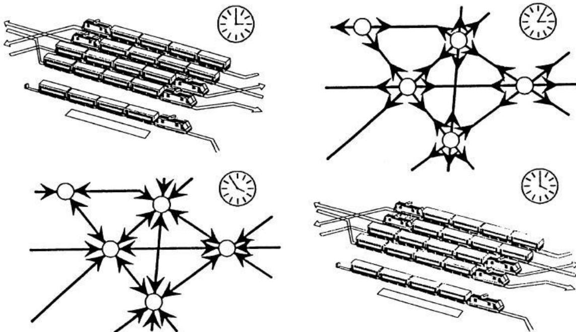
**Figure 2.2** Principle of IPT depicted by phases of symmetry time in IPT-node, departure of trains, arrival of trains and next symmetry time in IPT-node after one period (same minute) (Lichtenegger 1990).
