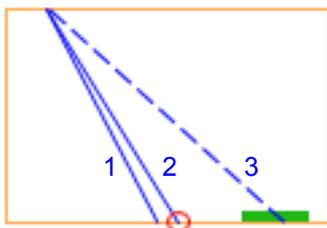
**Figure 3.9** Illustrations of various runtimes of a freight train: technical (1), regular (2) vs. system (3) runtime.
