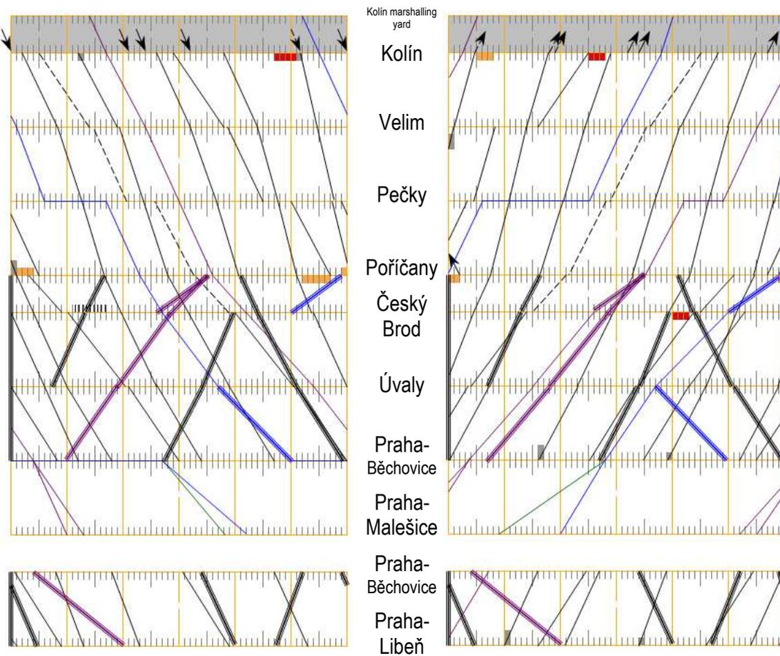
**Figure I.1** Proposed train diagram of PFTP for the line 501A/011.
