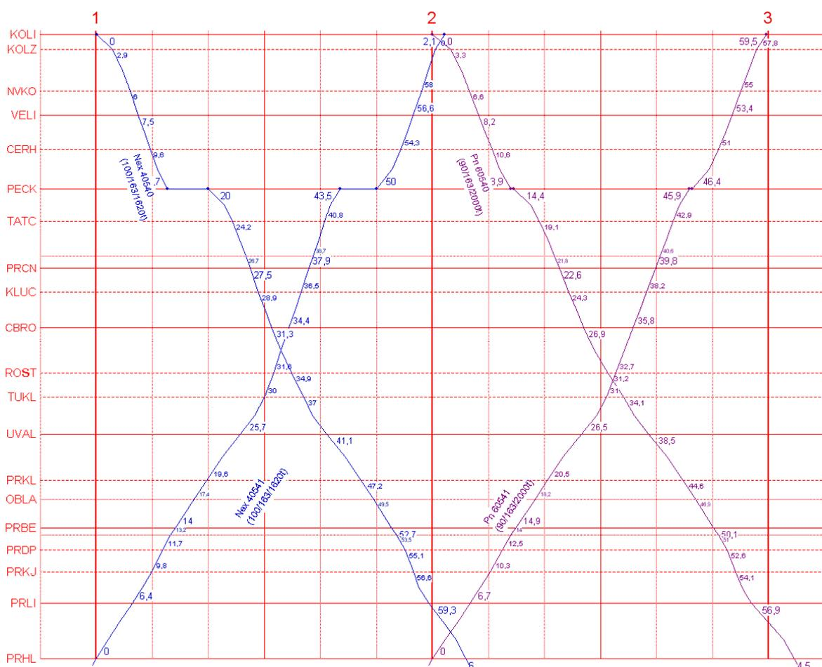
Figure F.1 Train diagram of model freight trains on the line 501A/011, section Kolín – Praha hl. n.
