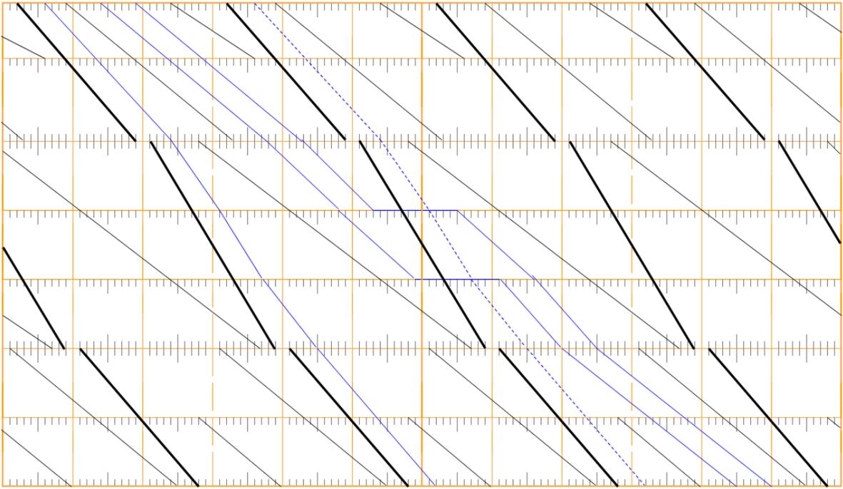
**Figure 3.18** Coordination with passenger transport: thanks to adjustment of regional trains, qualitative PFTP for express freight trains (marked by dashed line) can be constructed.
