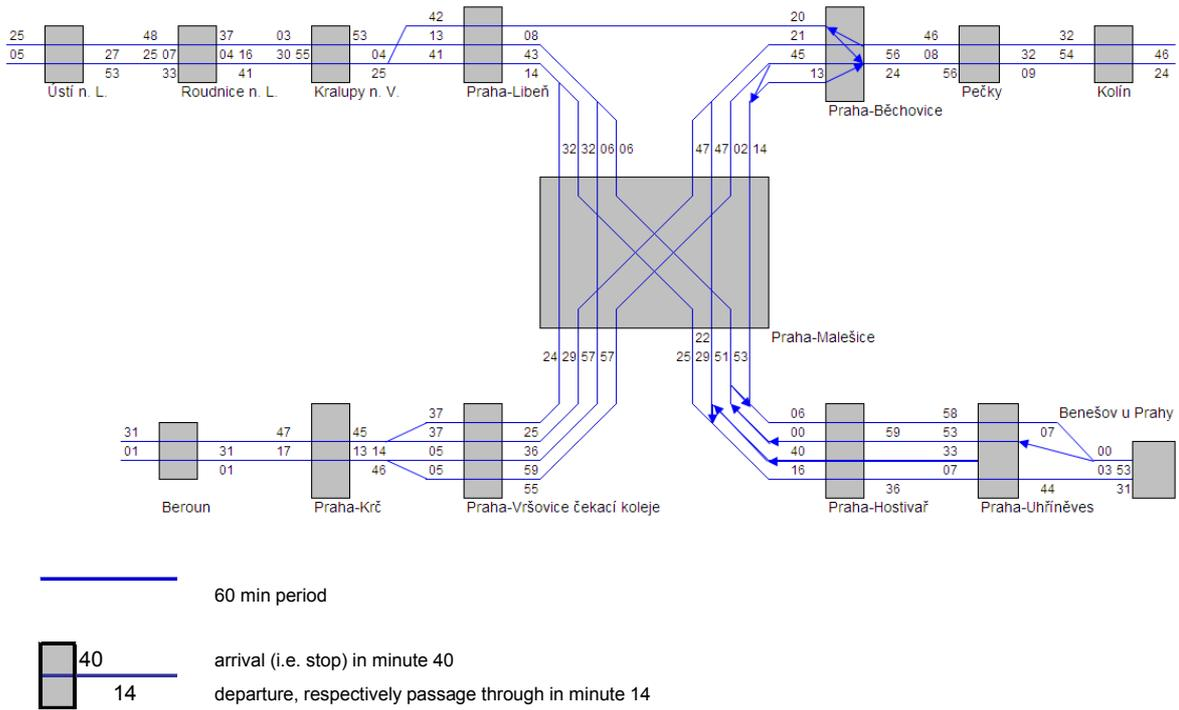
**Figure 4.3** Netgraph of PFTPs through Prague node area and adjacent lines (right-hand operation). Arrows stand for PFTPs in one direction only.
