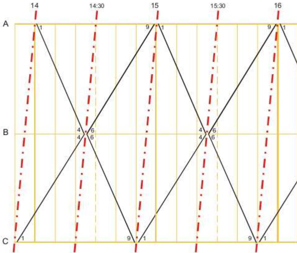
**Figure 3.12** Influence of asymmetric runtimes on symmetry time; symmetry time (axis) is marked by dot-and-dash. While there is zero symmetry in station A, in station C there is symmetry time in minute 50 (Kryže 2005).
