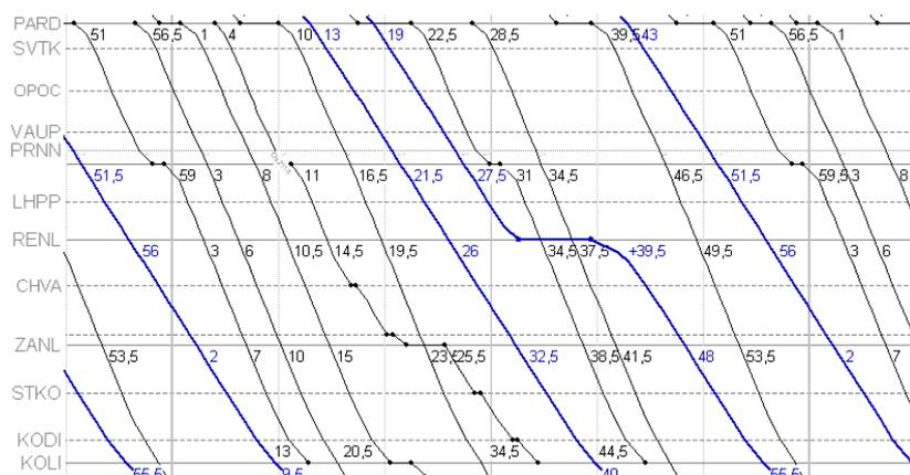
**Figure 4.8** Part of train diagram Pardubice – Kolín (one direction). Suggestion for coordinated solution for passenger and freight train paths (blue) (Kopecký et al. 2009, Drábek and Záruba 2010b).
