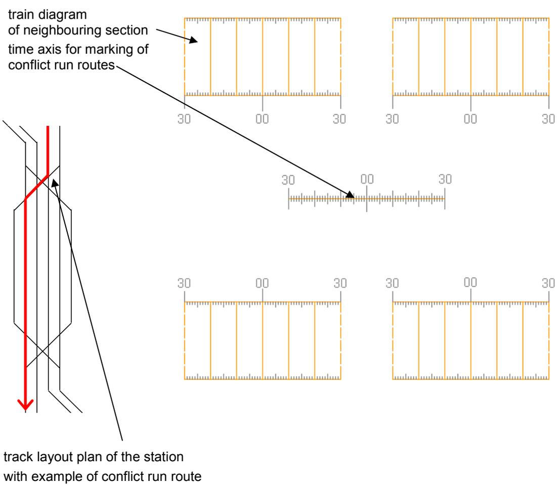
**Figure 3.13** Parts of node diagram.
