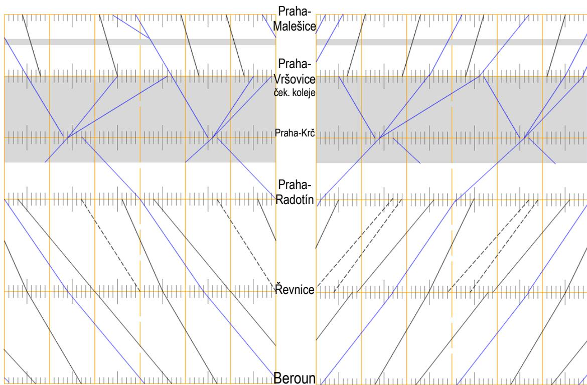
**Figure C.3** Proposed train diagram of PFTPs for the line 521A/171.
