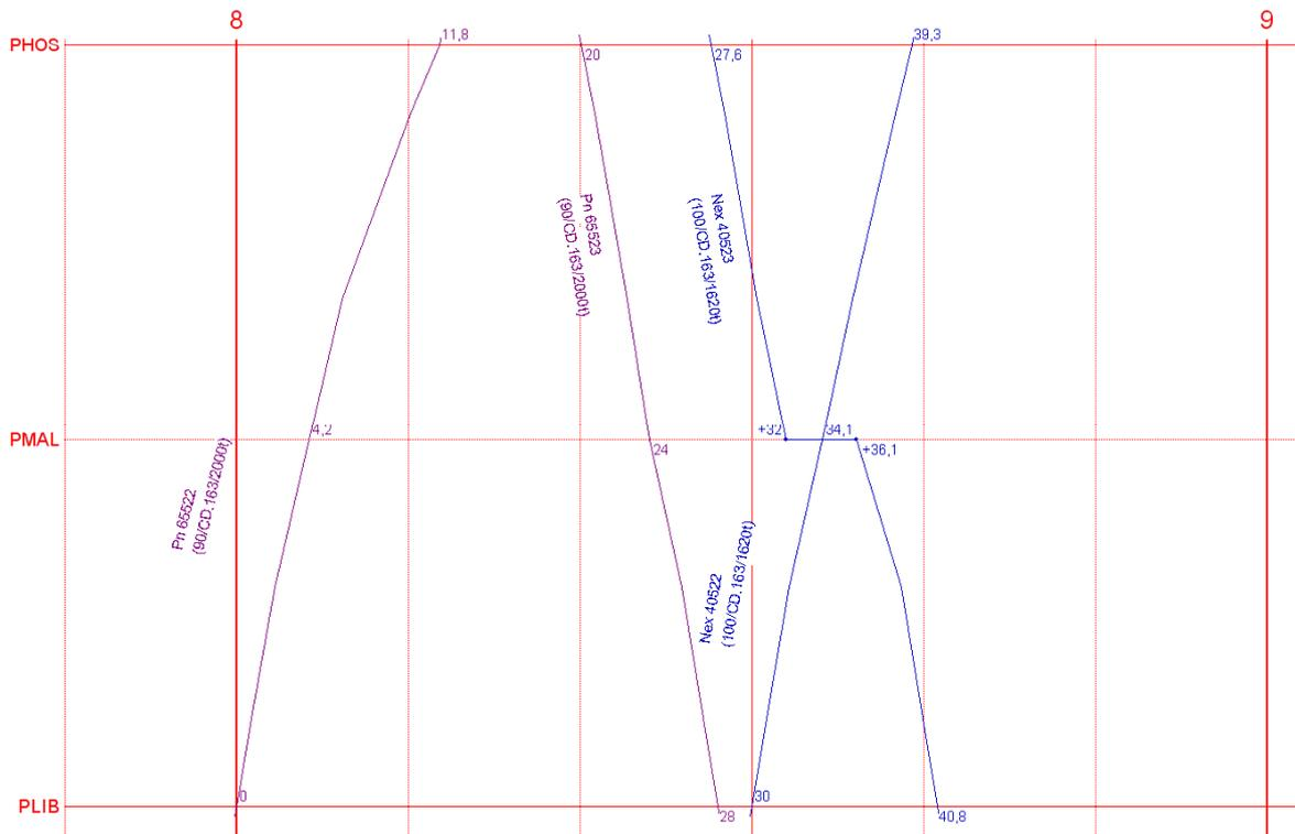
**Figure F.5** Train diagram of model freight trains on the freight bypass line 525F, section Praha-Hostivař – Praha-Libeň.
