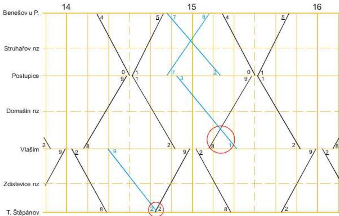
**Figure 2.8** Lack of usable capacity for freight trains on a local single-track line with periodic timetable of passenger transport. There are no block posts between stations. The freight train paths between Benešov u P. and Postupice are alternative. (Krýže 2005)
