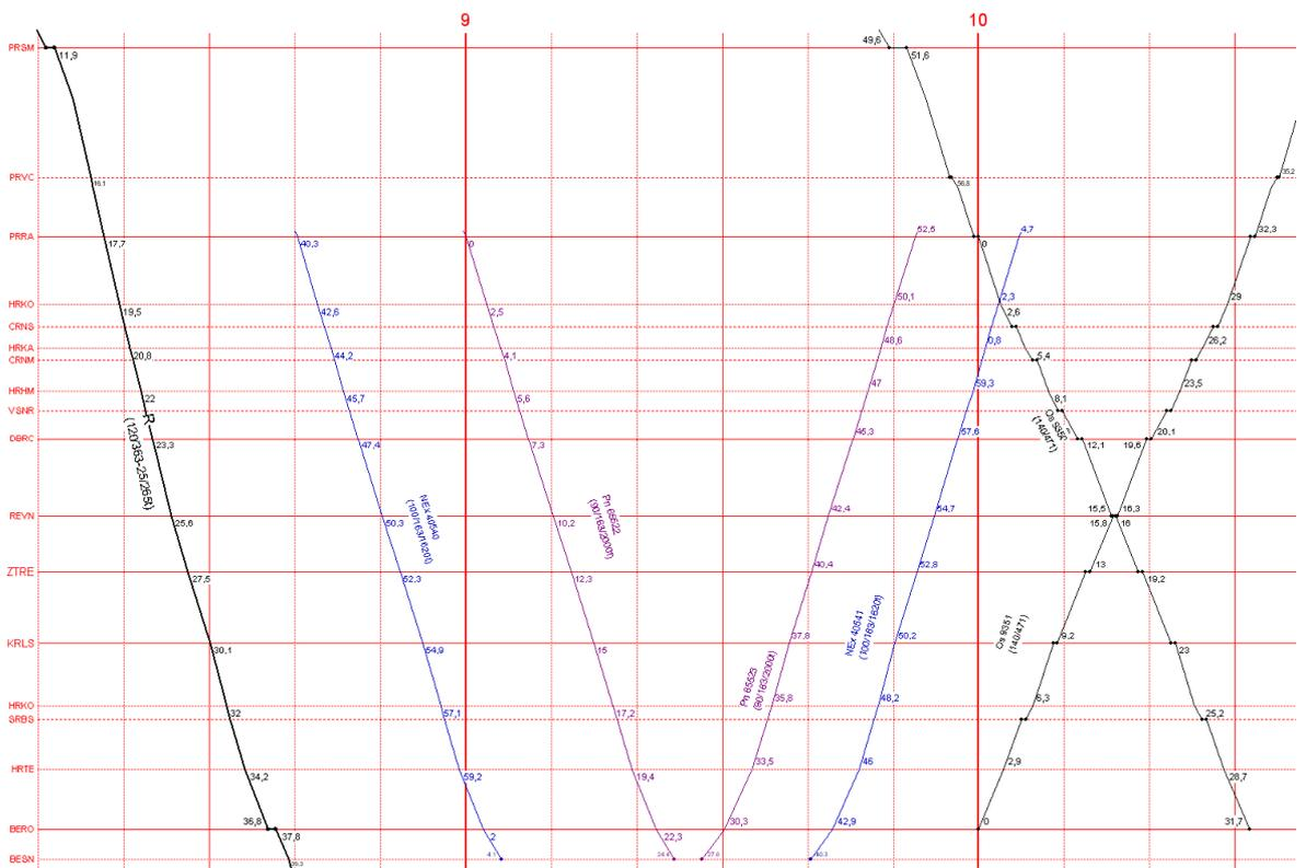
**Figure F.3** Train diagram of model freight trains on the line 521A/171, section Praha-Radotín – Beroun marshalling yard (Beroun seř. n.).
