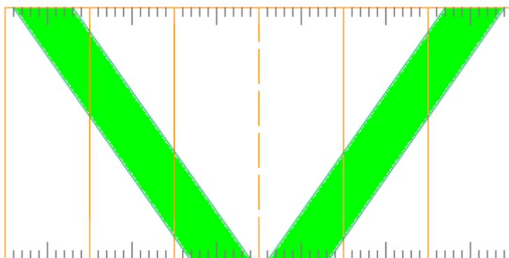
**Figure 2.6** Time windows for periodic train paths in the opposite direction on single-track line, if zero symmetry should be preserved.
