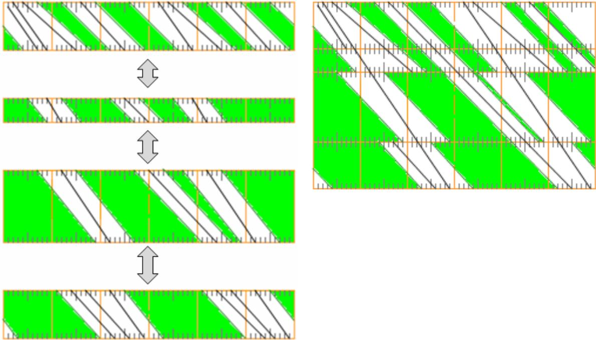
**Figure 3.10cd** Marking of usable capacity for freight trains in single sections and whole line – the usable capacity is delimited by passenger train paths, by minimal departure headways for passing through of a freight train and by minimal regular runtimes of freight trains
