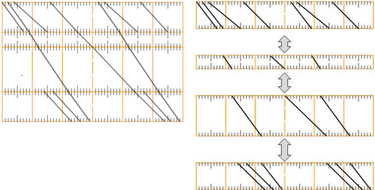
**Figure 3.10ab** Example of periodic passenger timetable in one direction (double-track line) and its division into sections with constant number and sequence of trains. The first and last sections are apparently bottlenecks of the line.
