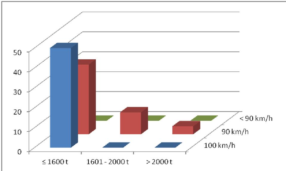
**Figure 3.4** Numbers of freight trains, scheduled through station Vlkov u Tišnova – overall 100 trains. 96% of them can run at 90 or 100 km/h and their brutto mass of load does not exceed 2000 t. Data: [SŽDC \(2009b\)](#)
