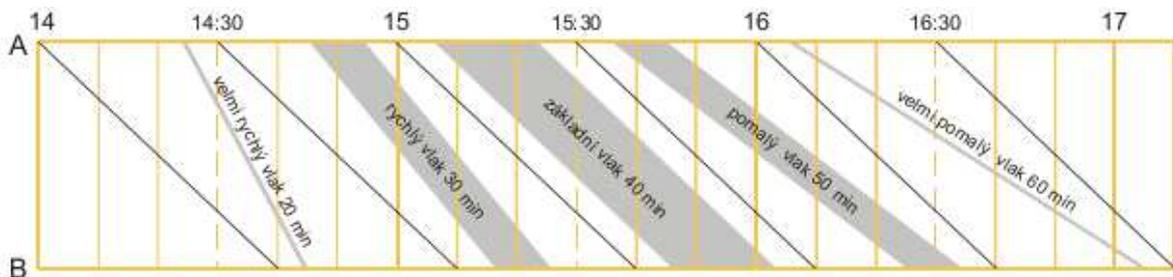
**Figure 2.5** Usable capacity (sizes of time window) for trains with different speeds in the context of periodic timetable on double-track line. Usable capacity for both “very slow” and “very fast” trains is very little. Slower or faster train cannot run through this section without overtaking ([Krýže 2005](#)).
