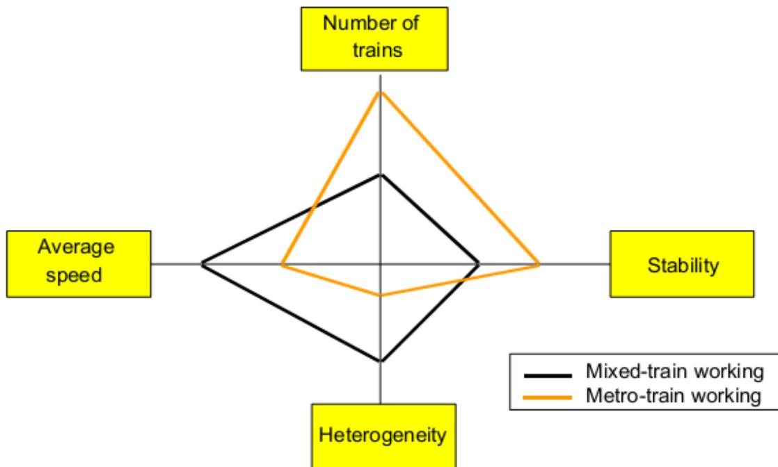
**Figure 2.4** Capacity chord – mixed and metro traffic (UIC 04).
