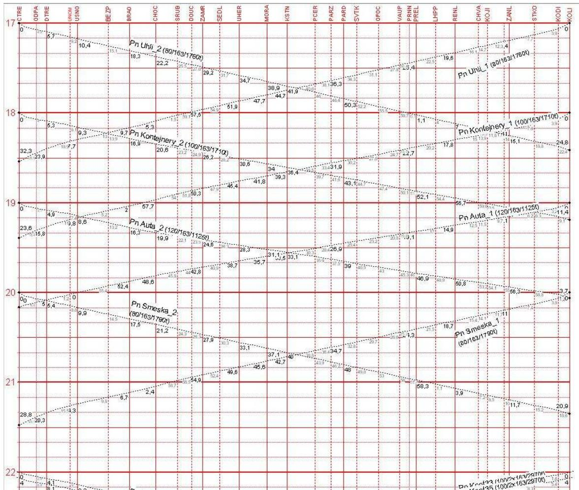
**Figure 3.5** Examination of suitability of periodic train paths for freight trains with same mass and locomotive, but different load, on main line section Česká Třebová – Kolín. From above, there is train pair with coal, containers, cars and wagonloads. In brackets there are maximum allowed speed/locomotive class/gross mass of load in tons.
