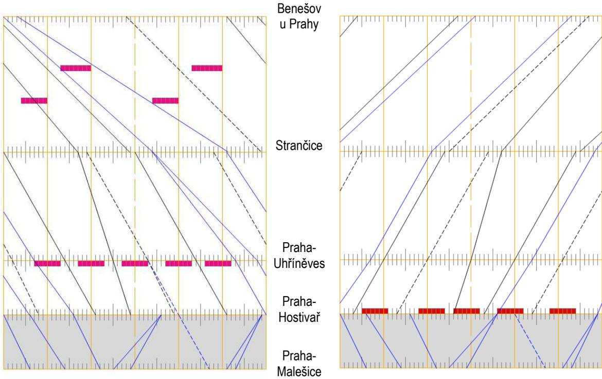
**Figure C.2** Proposed train diagram of PFTPs for the line 519A/221.
