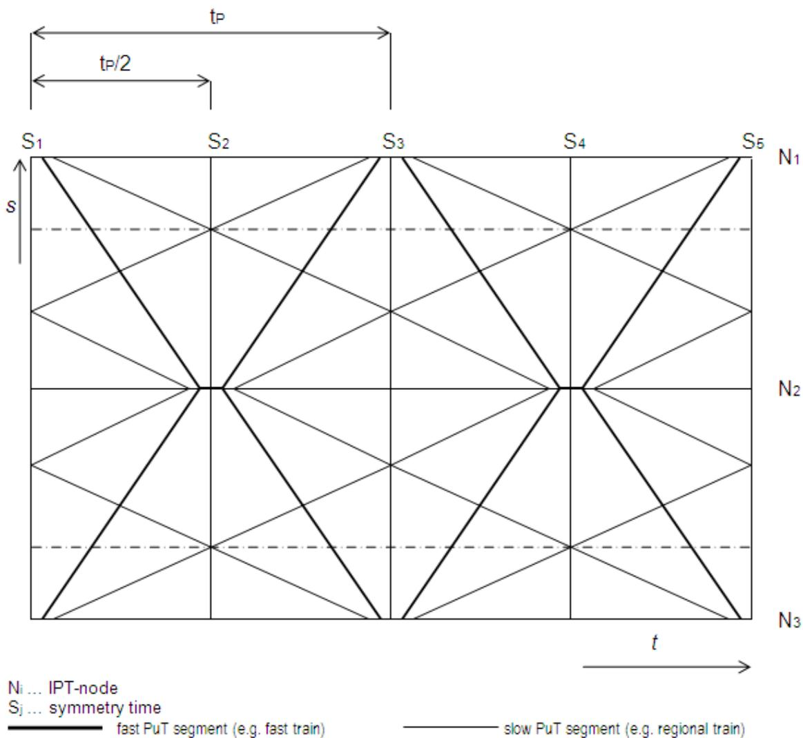
**Figure 2.1** Illustration of train diagram based on IPT, with marked basic period  $t_p$ , IPT-nodes  $N$  and periodically repeating symmetry times (symmetry axes)  $S$ . Adapted from [Baudyš \(2006\)](#).
